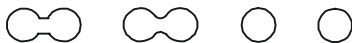
Fig. 4.1.4. Molecular bonding as two molecules move away from each other, the surface shape stretch, snap and finally contract into spheres.
