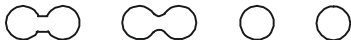
Fig. 8. Molecular bonding as two molecules move away from each other, the surface shape stretch, snap and finally contract into spheres.
